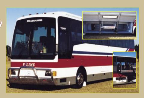
Cost effective dignified means of loading and unloading disabled peple. The cassette can be removed to maximise bin space and minimize weight and can be interchanged between similar set up vehicle therefore reducing capital costs
